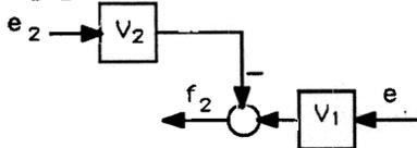
Figure 2:  $V_1$  and  $V_2$  describe the contributions of both inputs,  $e_1$  and  $e_2$ .
