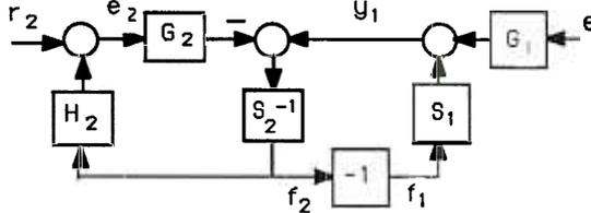
Figure 3: The Closed-loop System, the first robot controls the position and the second robot controls the force.
