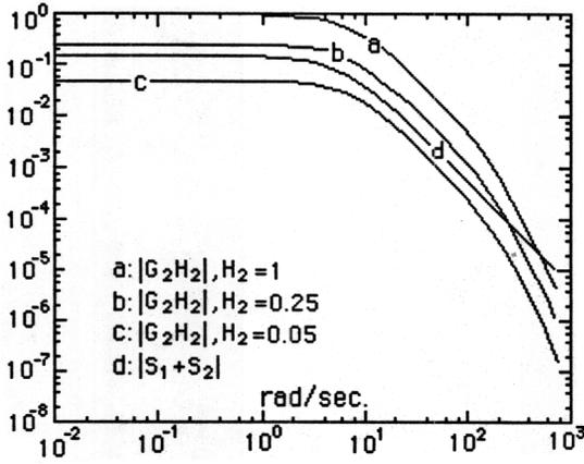
Figure 6:  $|G_2H_2| < |S_1 + S_2|$  is a sufficient condition for stability.
