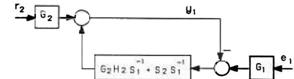
Figure B1: Simplified Block Diagram of the System in Figure 5
