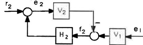
Figure 4: Two Manipulators with Force Feedback Compensator.
